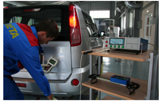
Multi-component gas analyser to measure CO, CO 2 , CH, O 2 , NO x concentrations, crankshaft rotation frequency during vehicle exhaust gases toxicity test AUTOTEST
